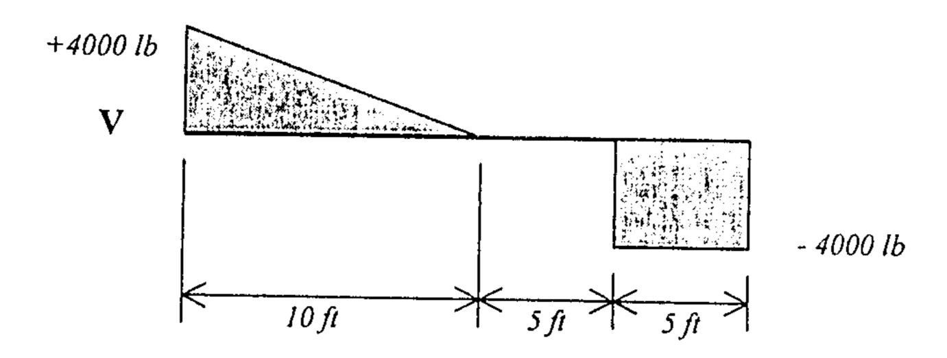
3. The beam of T-section is supported and loaded as shown in the figure. The cross section has width b=50 mm, height h=80 mm, and thickness t=10 mm. Determine the maximum tensile and compressive stresses in the beam.(25%)
