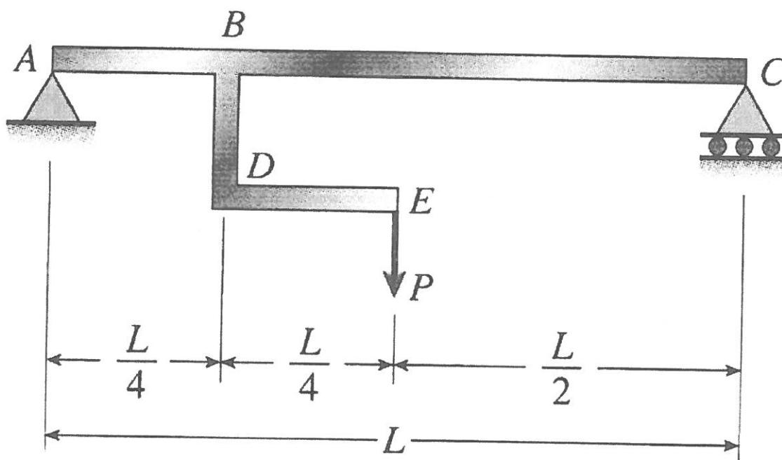
5. Determine the maximum moment and the corresponding location for the beam shown below. (20 pt)
