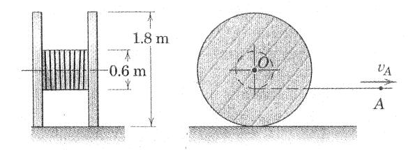
4. The 20-kg solid circular disk is initially at rest on the horizontal surface when a 12-N force P, constant in magnitude and direction, is applied to the cord wrapped securely around its periphery. Friction between the disk and the surface is negligible. Calculate the angular velocity  $\omega$  of the disk after the 12-N force has been applied for 2 seconds and find the linear velocity v of the center of the disk after it has moved 1.5 meters from rest.
