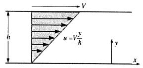
above. The flow is steady, incompressible, and two-dimensional in the xy-plane. The velocity
