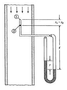
$$\frac{P_1}{\gamma} + z_1 + \frac{{V_1}^2}{2g} = \frac{P_2}{\gamma} + z_2 + \frac{{V_2}^2}{2g}$$
