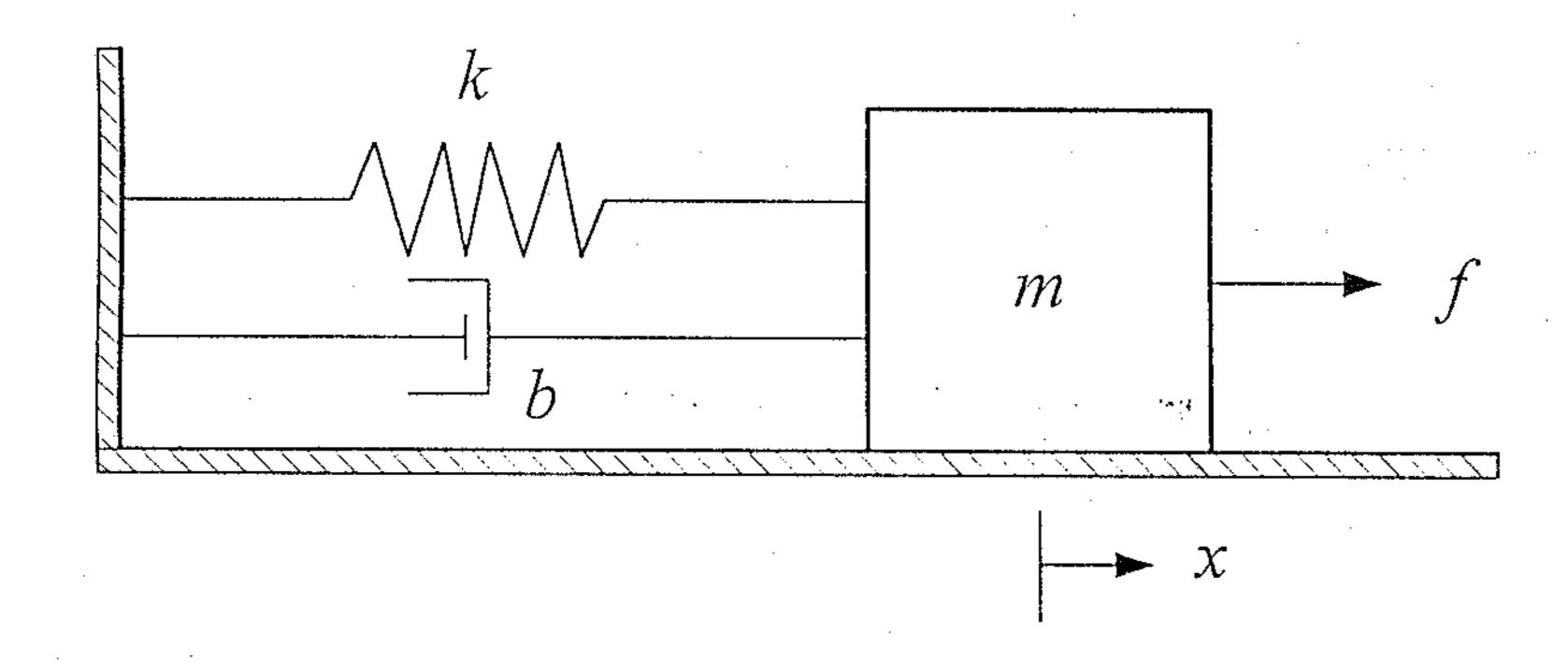
where f is the force applied to the mass, k is the spring constant, b is the friction constant, m is the mass, and x is the displacement of the mass. From force balance, the dynamics of the mass-spring damping system can be written as
