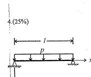
A simply supported beam is subjected a uniform load p. The deflection curve v(x) satisfies the differential equation
