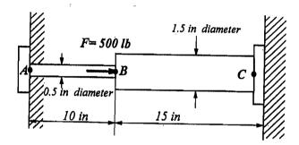
A step shaft (shown below) transmits a torque of 3000 lb-in. Determine the
