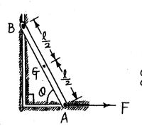
A constant force F=4N is applied to a uniform slender rod which is initially at rest in the  $\theta=90^{\circ}$  position. The rod has a length  $\ell=500$ mm and a mass m=0.3kg. Center of mass of this rod is at G.
