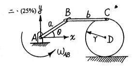
Link AB has a length a=400mm, and link BC has a length b= 600mm. The circular disk has a radius r=250mm which rolls without sliding on the ground. At the instant shown in the figure,  $\theta$ =30° and link AB rotates with an angular speed  $\omega_{AB}$ =0.5rad/sec. Determine velocity  $v_C$  of joint C, angular velocity  $\omega_{BC}$  of link BC, and angular velocity  $\omega_{CD}$  of the circular disk.
