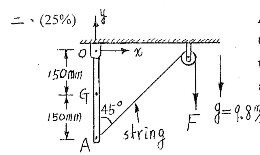
A 0.4kg slender rod, originally at rest, is pulled by a force F=0.8Nt. Center of mass of this rod is at G. Draw free body diagram of this rod and determine reaction forces at O, and angular acceleration  $\vec{\alpha}$  at this moment.
