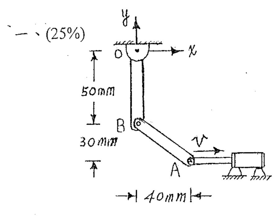
The piston of the hydraulic cylinder gives pin A a constant velocity v=200 mm/sec at this moment.
