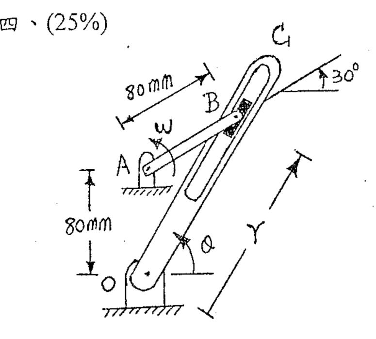
At the position shown in the figure, link AB rotates with a counterclockwise angular velocity  $\omega = 5$  rad/sec.
