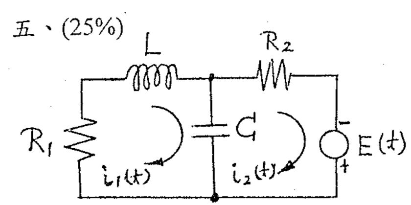
Using electrical charges as variables, obtain equation(s) of motion for the circuit shown in the figure.
