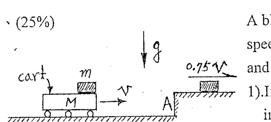
A block of mass m moves together with a cart of mass M with a speed v. After striking with an obstacle at A, the cart stays at A and the block moves further with the speed 0.75v.
