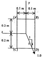
2. Plot the shear force and bending moment diagrams for the beams shown in the figures. (15%).
