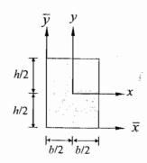
$I_x = bh^3/12$ ,  $I_{\bar{x}} = bh^3/3$  $I_y = b^3h/12$ ,  $I_{\bar{y}} = b^3h/3$
