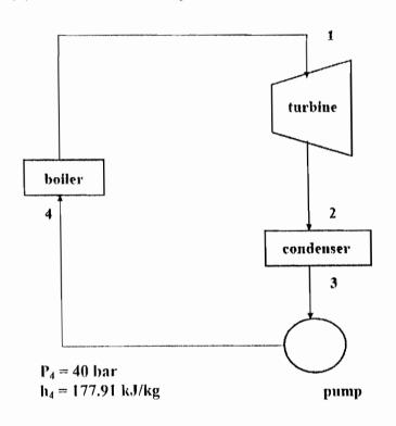
$P_1 = 40 \text{ bar}$   $T_1 = 480 \, ^{\circ}\text{C}$  $h_1 = 3399.2 \text{ kJ/kg}$
